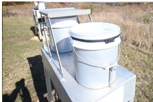
Figure 6. Seal the previous weeks sample bag bucket. Aerochem (left) and NCON (right).
