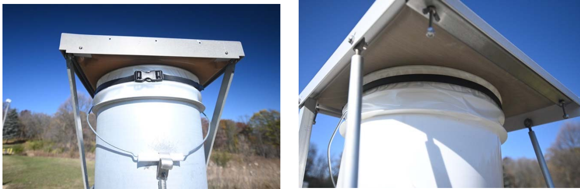
Figure 12. Check the lid pad seal on the sample bag bucket. Aerochem (left) and NCON (right).
