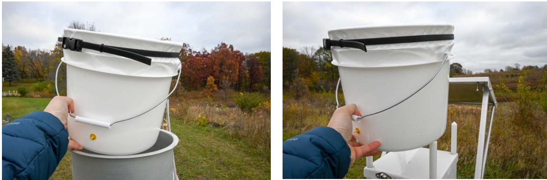
Figure 11. Place the new sample bag bucket on the Aerochem (left) or NCON (right) collector.
