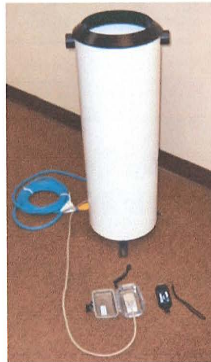
Gauge, SC115 Cable and Box
