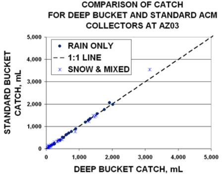
**Figure 4.** Comparison of catch efficiency for deep-bucket and standard bucket Aerochem Metrics precipitation collators at NTN site AZ03.
