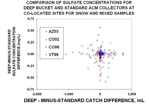
**Figure 6.** Variation of sulphate concentration differences for collocated deep-bucket and standard bucket Aerochem Metrics collectors for weekly samples containing frozen precipitation.
